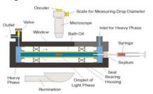
A droplet located along the axis of a rotating capillary filled with denser fluid will form a cylindrical shape. With the appropriate drop volume and rotational speed, the drop diameter depends solely on the interfacial tension. The droplet stabilises in the axis of rotation, while the surrounding fluid is forced outward owing to its higher density.
