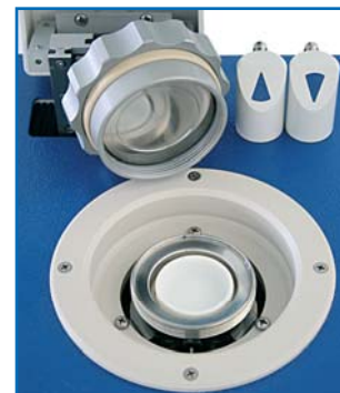
stainless steel chamber with PTFE-sample dish
