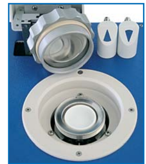
stainless steel chamber with PTFE-sample dish
