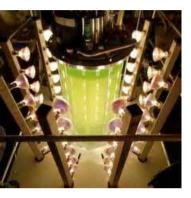
Diachrom Biotechnology Photobioreactors DIAPBR, is a device that can contain and grow algae, cyanobacteria and other photosynthetic organisms under heterotrophic and mixotrophic conditions. Our PBR system is a controllable environment in which to grow algae, and where the supply of light, nutrients, carbon dioxide, air, and temperature can be controlled and regulated.
