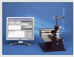
Automatic image analysis simplifies the measurement of extremely low interfacial tensions with the Spinning Drop Tensiometer SITE100. Excellent temperature control and optimum synchronization of the instrument allow the sample to be observed over a long period of time at constant conditions.
