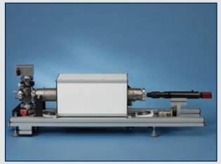
The high temperature measuring places of DSAHT serial stands out with the simplest sample change, excellent contour analysis and user friendly operation. We use the modularity of the measuring system to meet the special requirements of various applications and temperature range.
