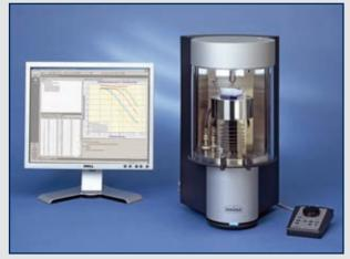
The BP100 measures the dynamic surface tension of liquids using the maximum bubble pressure method. Fast wetting and dewetting processes can thus be fine-tuned according to application. The whole measuring process is controlled with a PC. The data will be collected, displayed and if necessary used for further evaluation.
