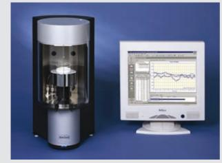
The Single Fibre Tensiometer K100SF is the process-controlled measuring system for the exact characterization of single filaments. Extremely high measured value resolution combined with the high precision of the mechanical components predestines the K100SF for measuring fibres
