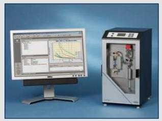
The Drop Volume Tensiometer DVT50 allows the interfacial tension between two liquids to be measured, at a variety of interface ages. At the same time, the DVT50 offers fully automatic measurement for dosing speeds and temperatures.
