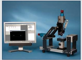
The nondestructive contact angle measurement in recesses and on strongly curved surfaces in combination with the high measuring accuracy of very small contact angles make the TVA100 unique.
