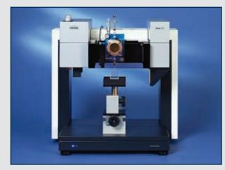
Interfacial rheology is a crucial parameter for the formation and stability of foams in particular. With the DSA100R the elasticity of the interfacial film can be determined both optically and by capillary pressure measurement.
