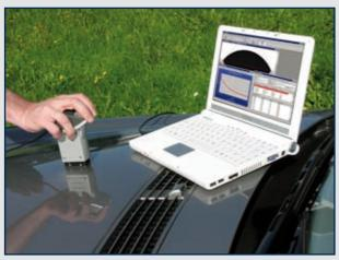
With GH11 the user can measure contact angle, surface energy on-site and network-independent. The GH11 can be used as an ideal quality control tool because of its extreme simple handling, portability and small size.
