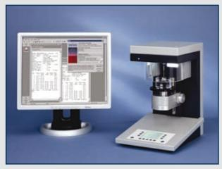
The Digital Tensiometer EasyDyne (K20 / K20S) is the reliable companion for professional users who only have to measure surface and interfacial tension occasionally. The EasyDyne can also be used for measuring at controlled temperatures.
