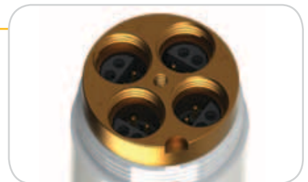
EXO1 sonde contains 4 universal sensor ports
