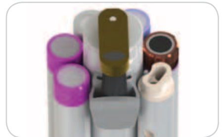
Wiper keeps sensors clear of biofouling
