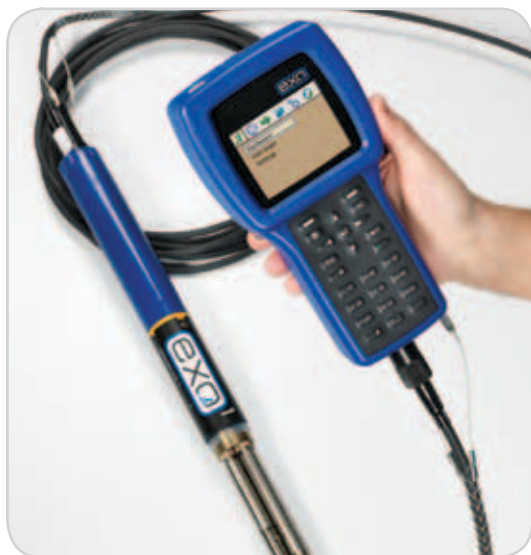
Interface with the EXO Sonde using the EXO Handheld Display
