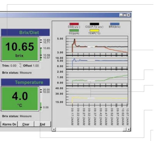
Large numeric displays for each parameter, with color-coded background to indicate alarm conditions.
