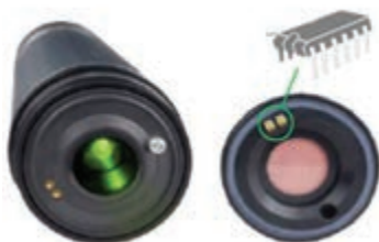
Sensor cap with memory chip for calibration data
