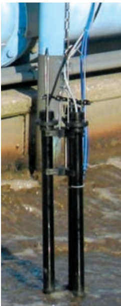
With extensions and triple sensor holder
