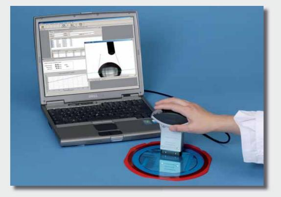
MobileDrop is a semiautomatic and fully integrated system for measuring contact angles and surface free energies on samples of virtually any size. Its low weight, operation with a notebook and simple handling mean that the instrument is a flexible and reliable partner for quality assurance, both in the lab and on-site.
