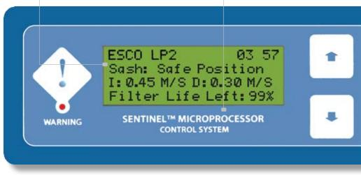
When programmed ON • the start-up sequence confirms status with Air Safe and local time display.
