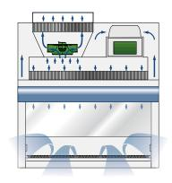
**1A:** Under normal operation with both fans operating (1a) the supply fan creates a negative pressure surrounding the contaminated positive pressure plenum and pushes air across the supply and exhaust filters. The exhaust fan boosts the air pressure through the exhaust filter to create better inflow and operator protection. Supply and exhaust fans automatically operating at reduced speeds extend fan life.
