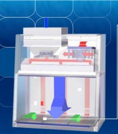
ULPA-filtered air Unfiltered / potentially contaminated air Room air / Inflow air
