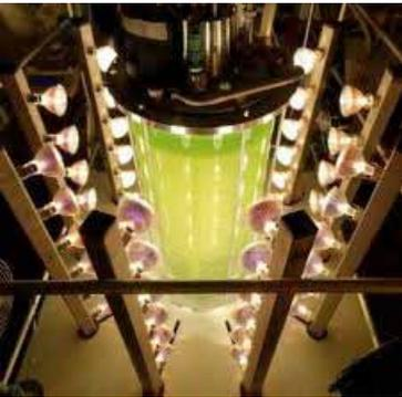
Diachrom Biotechnology Photobioreactors DIAPBR, is a device that can contain and grow algae, cyanobacteria and other photosynthetic organisms under heterotrophic and mixotrophic conditions. Our PBR system is a controllable environment in which to grow algae, and where the supply of light, nutrients, carbon dioxide, air, and temperature can be controlled and regulated.
