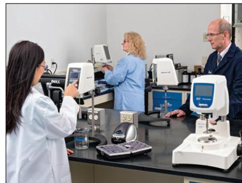
AMETEK Brookfield's state-of-the-art laboratory offers a variety of viscosity testing services capable of measuring Newtonian and non-Newtonian fluids using a wide range of spindle geometries. Detailed test results include equipment and measurement system description, viscosity data which includes appropriate tables and graphs, and any recommendations pertinent to your specific material and associated method.
