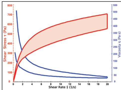
**Thixotropy Analysis:** up/down shear rate ramp produces curves for shear stress vs. shear rate (red color) and viscosity vs. shear rate (blue color). Thixotropy calculation is the area between the red curves, approximately 2,000 Pa·s.
