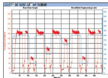
*Test algorithm for AMETEK Brookfield PFT requires compression of the sample contained in an annular shear cell to defined axial loads followed by torsional shearing to determine powder failure strengths.*
