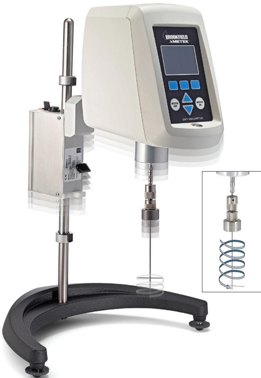
For viscosity/consistency measurement of gels, pastes, creams, putty, gelatin and other non-flowing substances.
