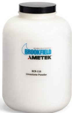
*To perform a calibration check on your Powder Flow Tester, use certified BCR-116 limestone powder. Run the standard Flow Function test at 5 consolidation stresses and record the failure strength values. They must be between published min/max values for the instrument to pass. BCR-116 limestone powder is supplied in 3.2kg jars and certified by the European Commission, Community Bureau of Reference. Contact AMETEK Brookfield for more information.*
