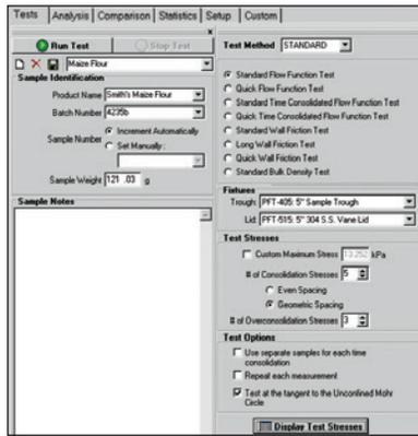
Main screen provides choice of basic tests:
