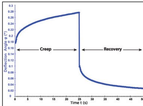
**Creep /Recovery Behavior:** material flow under constant stress is measured by detecting angular rotation of spindle; when constant stress is removed, recovery is measured by backward rotation of spindle.
