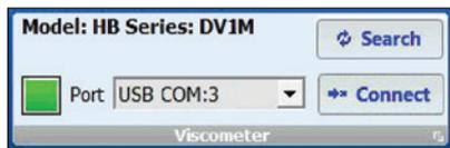
The DV1 Viscometer communicates to the PC through USB A port. The interface cable is supplied with Wingather SQ Software. Successful communication is indicated by a green light beside the port designation.
