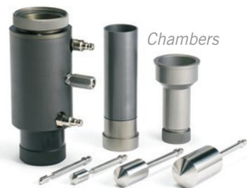
*Coaxial Cylinder Spindles*
