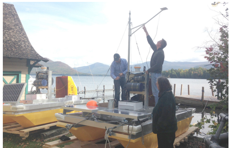
YSI applications specialists and customer set up a Vertical Profiler
