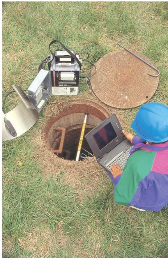
The 4250 Area Velocity Flow Meter is ideal for sites where submerged, full pipe, surcharged, or reverse flows may occur.
