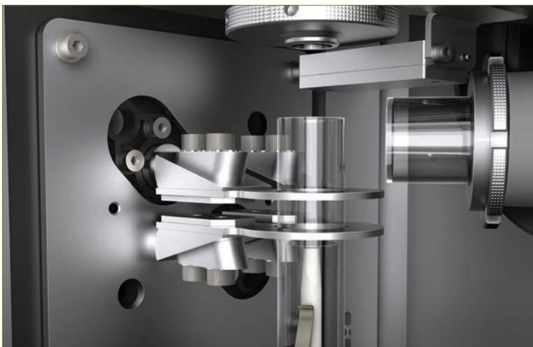
Avio's proprietary Flat Plate plasma technology provides a more compact, robust, and stable plasma than traditional helical coil systems.
