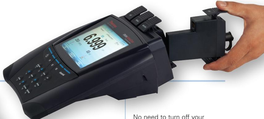
No need to turn off your meter to switch modules – meter automatically recognizes module changes.
